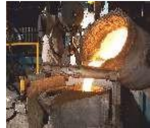
A large pump component being poured.
