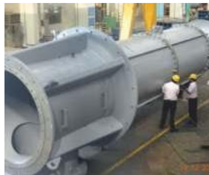
Termozulia Power Project, Maracaibo, Venezuela Two Circulating Water Pumpsets for 480 MW Power Project
