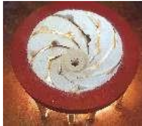
An impeller core of a large pump is being set in the mould.
