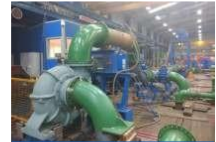
Factory Test Set-Up For 1 x 65 kW PAT for Shatin WTP Hongkong
