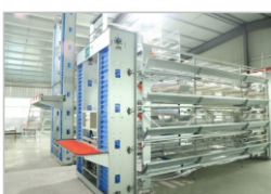
H-Layer Battery Cages
