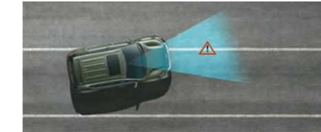
alerts the driver whenever the car is going out of its lane on either side without turn indicator input
