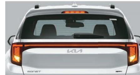
alerts the driver behind by blinking the brake lights whilst braking sharply and severely
