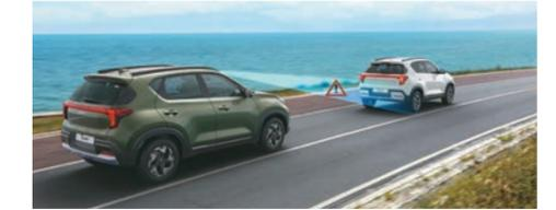
alerts the driver of imminent collision with the car ahead and applies brake
