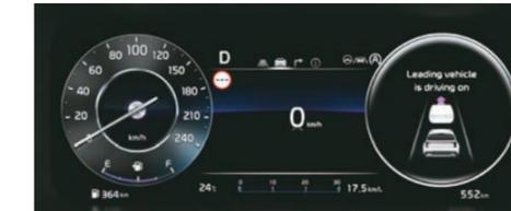
informs the driver if the vehicle in front starts moving and driver does not react
