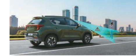
alerts the driver of imminent collision with any pedestrians ahead and applies brake
