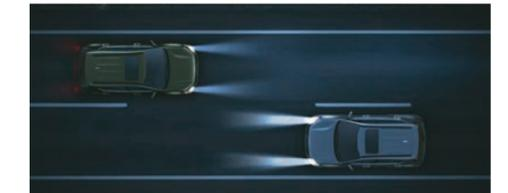
automatically adjusts the high beam/ low beam based on the oncoming vehicle's headlamp intensity
