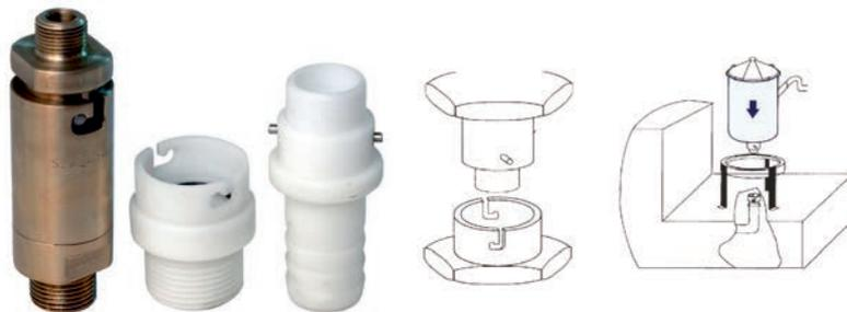
Pin lock system is designed as a alternative to a ball lock system for typical application. This system facilitates use of only one hand to connect or disconnect & so can be effectively used where the connection points is in a closed or difficult to reach position. This system is also useful for flow of powder & slurry. In ball lock, solid particles can enter locking ball mechanism restricting the movement of balls making the connection & disconnection difficult.
