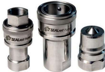
These couplings have automatic shut off valve at both ends; in socket & plug also. So on disconnection both socket & plug are sealed instantly. This type is widely used on Hydraulic lines carrying oils, water, chemicals & petroleum products. Material & seal are selected to suit the type of fluid.
