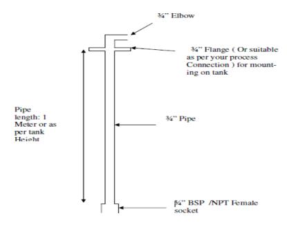
MOC of Pipe / Socket / Flange : SS304 / SS 316 / PP / PVC as per Application Note: Fabricate the dip pipe in a way that pH sensor should always dip in solution
