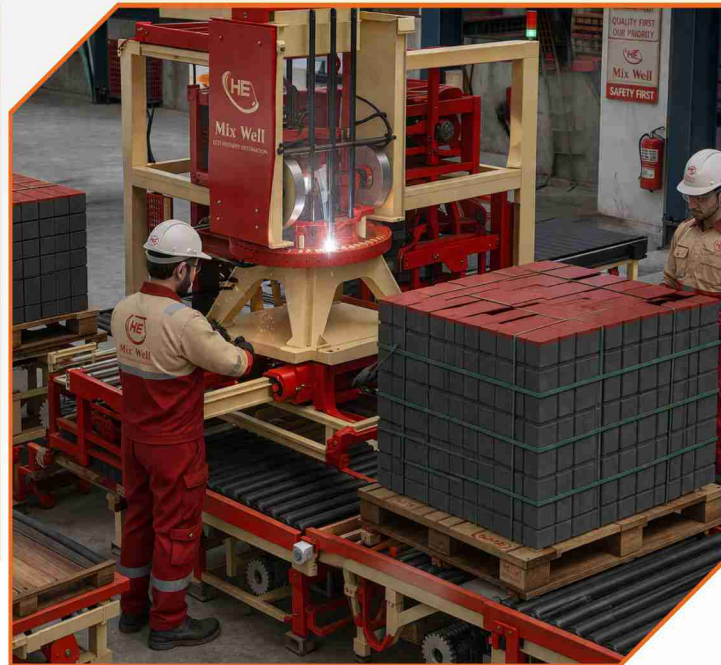
CUBER (BRICKS HANDLING SYSTEM)
