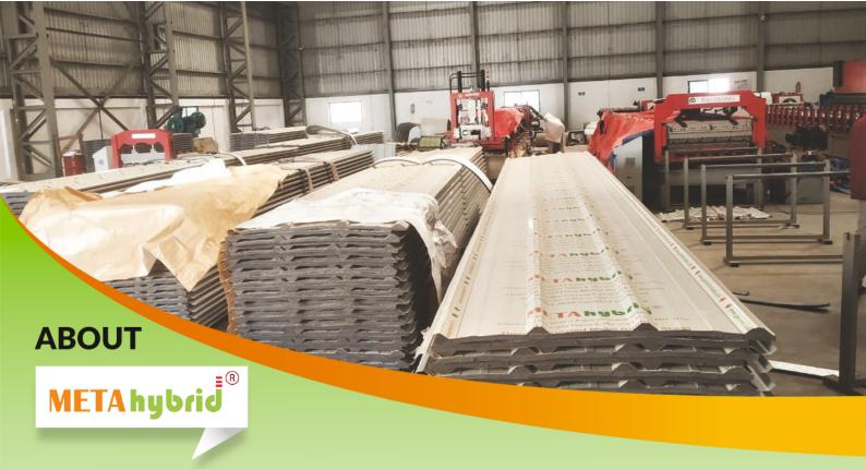
Is a unique Thermal Insulated metal roofing sheets solution developed by GEOMETRIC STEELS. An under-deck multilayer thermal insulated metal roof and wall cladding sheet. It has a unique composition of thermal insulating material as per application and customer's needs.
