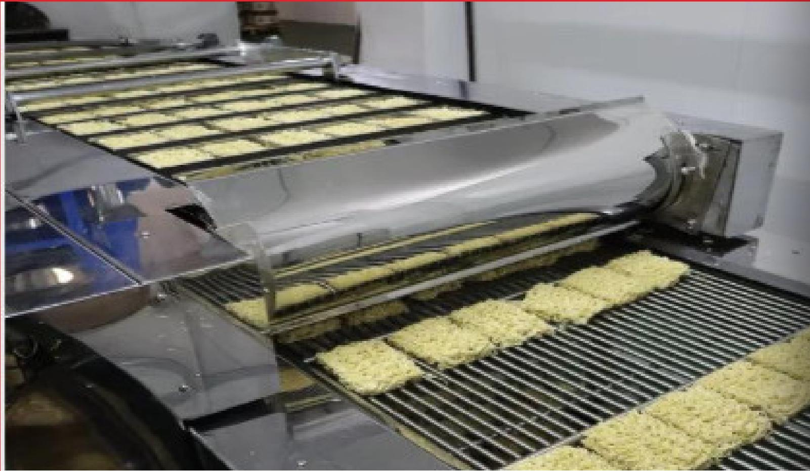
An automatic Maggi cutting machine is a specialized piece of equipment designed to efficiently cut and fold steamed noodle sheets into uniform blocks, essential for high-volume instant noodle production. These machines are integral to the manufacturing process, ensuring consistency and quality in the final product.
