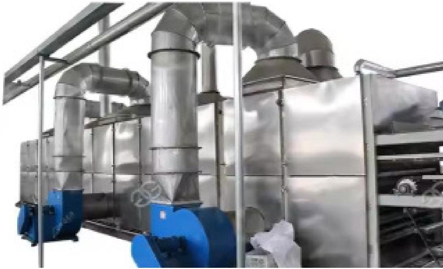
**A continuous dryer for Maggi-style instant noodles is a vital component in the production line, particularly for non-fried (hot-air dried) noodles.**
