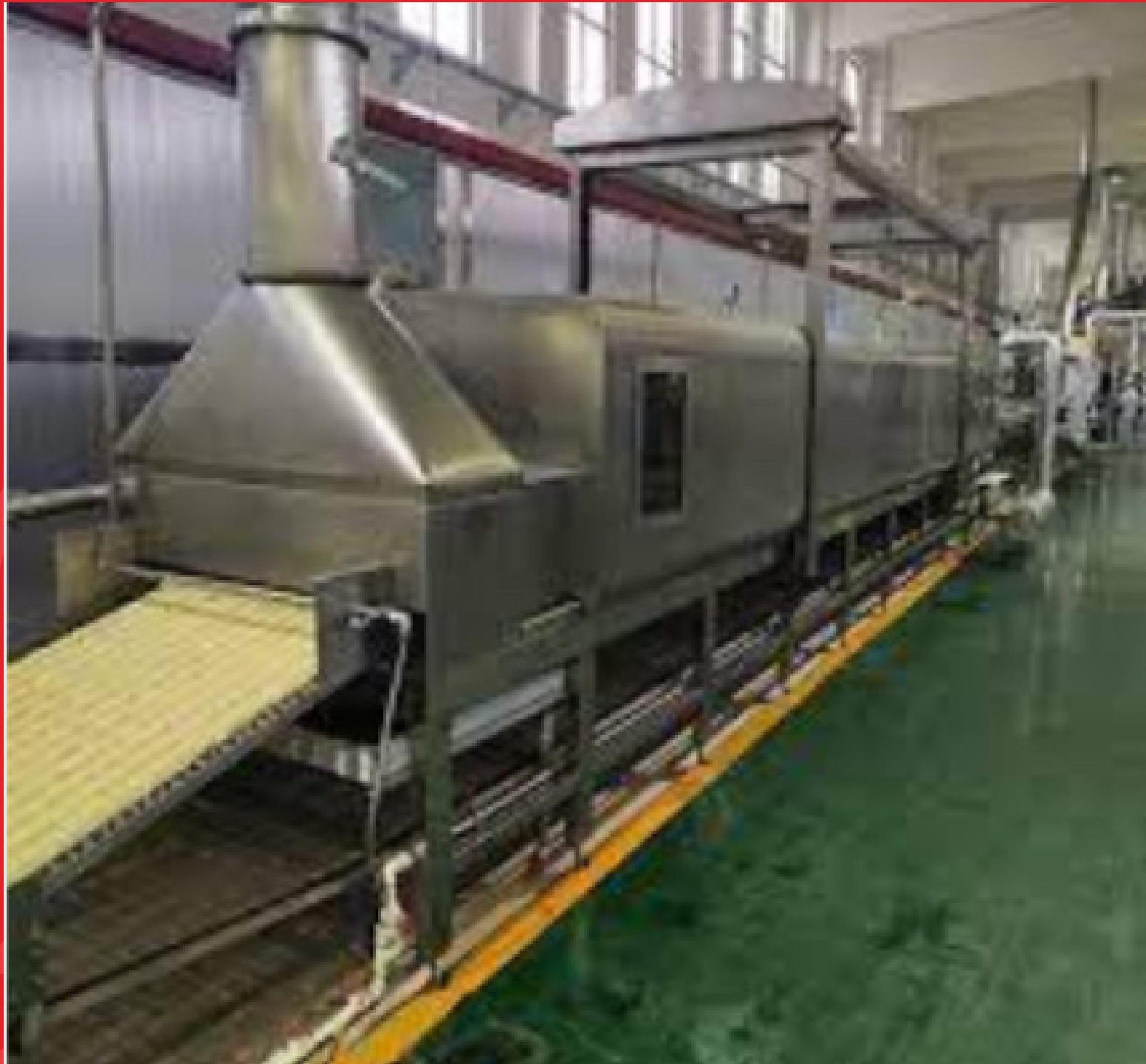
An instant noodle steamer with a gas burner is a specialized piece of equipment designed for the efficient steaming of noodles in high-volume production settings. These steamers are integral to the noodle manufacturing process, ensuring that the noodles achieve the desired texture and quality.
