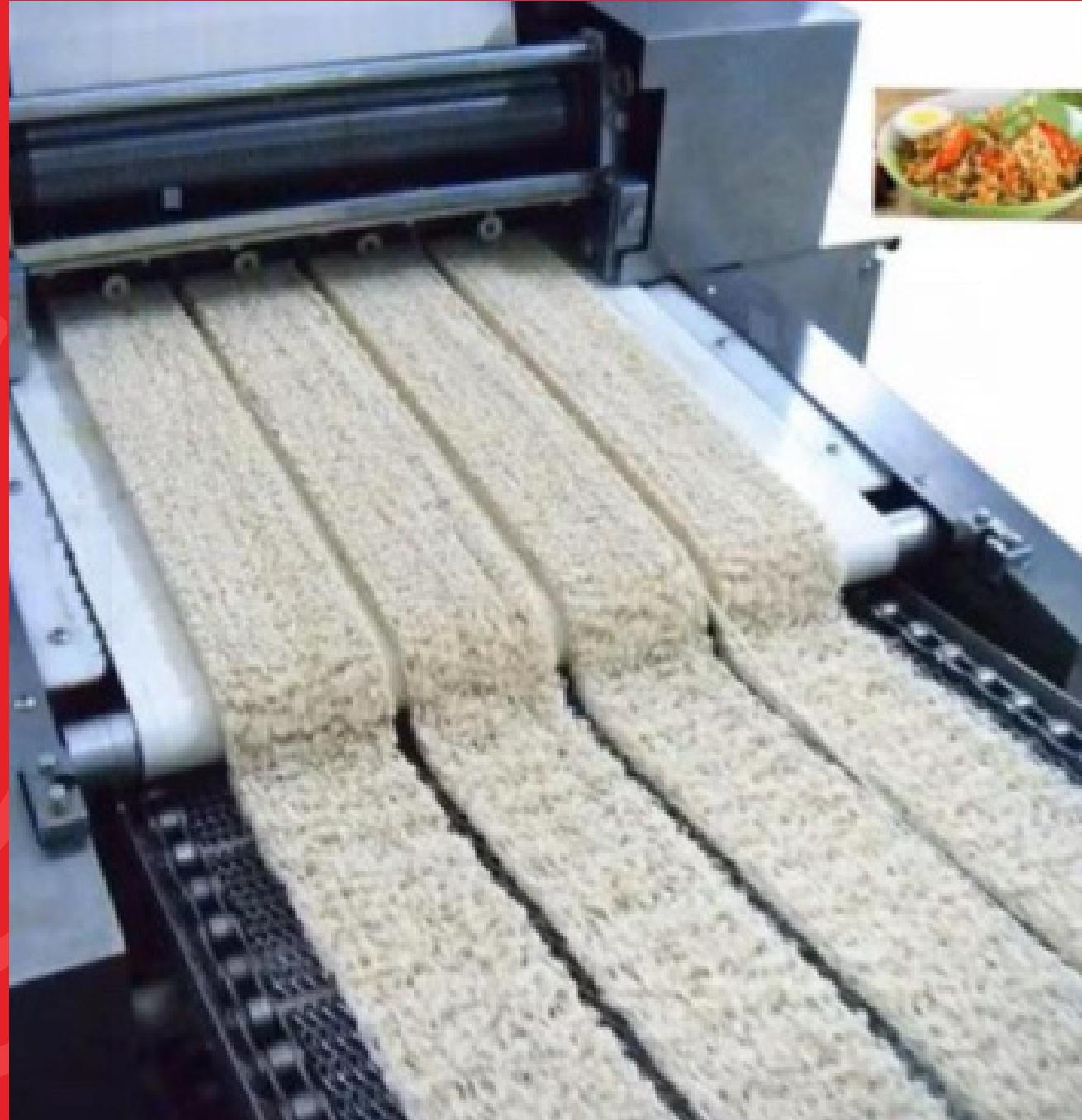
**The instant noodle rolling and cutting system is a crucial component in the production line, transforming dough into uniform noodle sheets and shaping them into the desired form.**
