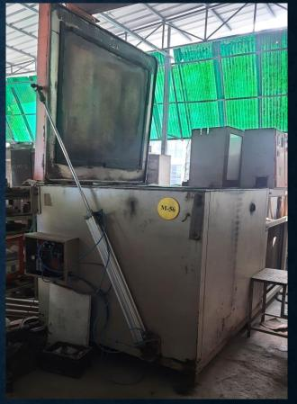
SQF with Integrated Quenching Tank, Fully Computerized SCADA Controls, And Sub-Zero Treatment
