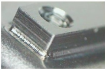
Inside Corner Seam Welding
