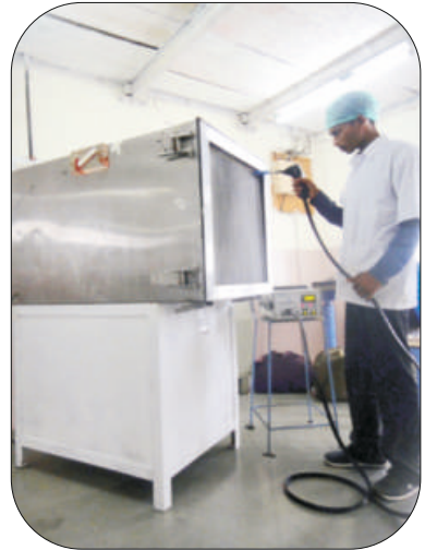
Leakage Test Rig (as per IEST-RP-CC0034)
