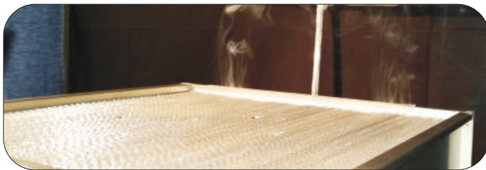
Oil Thread Test Rig (also known as Visual Leakage Test Rig)
