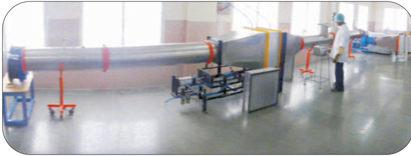
Efficiency Test Rig (based on EN 1822)
