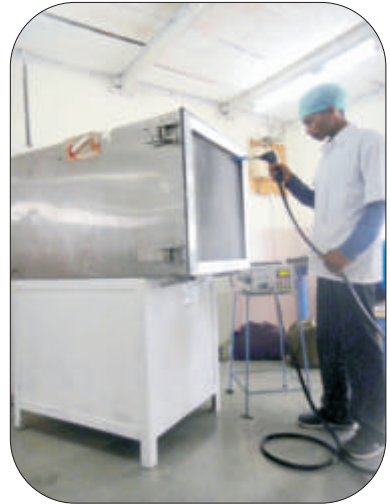
Leakage Test Rig (as per IEST-RP-CC0034)
