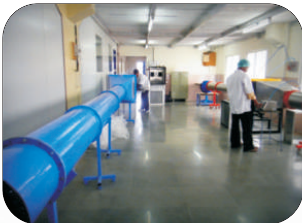
Over Pressure Test Rig (as per BARC specs.)
