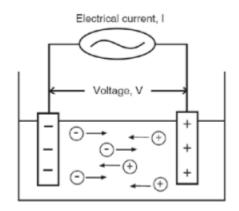
The resistance of the solution (R) can be calculated using Ohm's law as shown below. The resistance unit is [Ohms] or  $[\Omega]$ .
