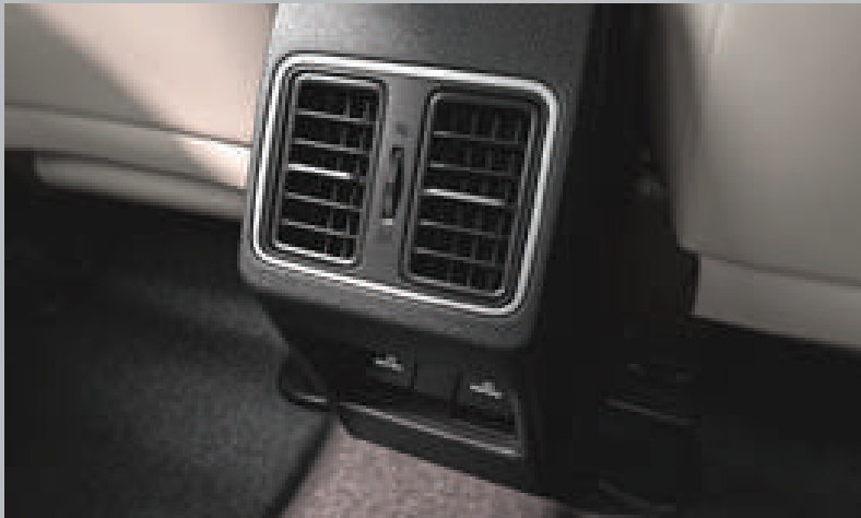
REAR AC VENTS WITH CHARGING PORTS (2)
