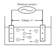
The resistance of the solution (R) can be calculated using Ohm's law as shown below. The resistance unit is [Ohms] or  $[\Omega]$ .
