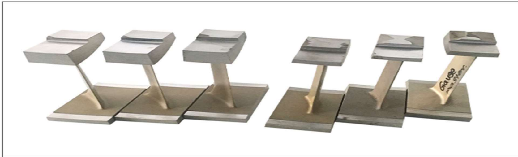
High Pressure and Low Pressure Aeroengine Vanes (Material: Aluminium Alloy)
