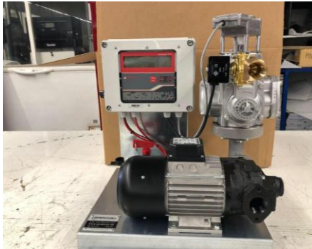
Compact Mobile Fuel Transfer Skid
