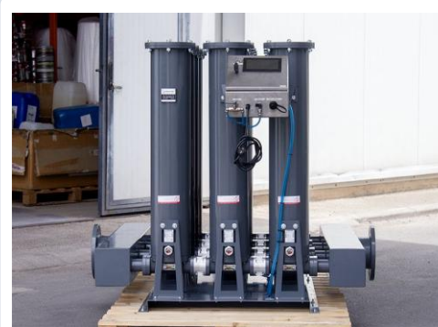
3-stage Filtration Unit With Particle Counter
