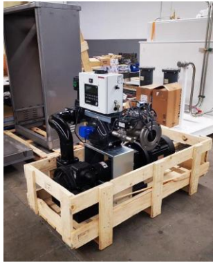
Digital BMS Integrated Fuel Unloading Skid
