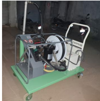
Light Aircraft Refueling Skid
