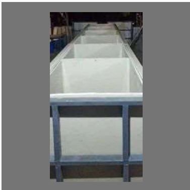
Pp Pickling Tank
