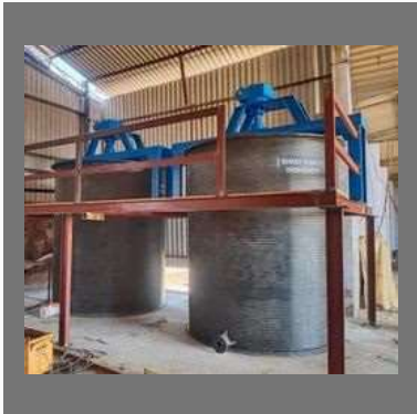
7500L HDPE Open Reaction Vessel
