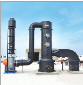
Wet Scrubber System is designed to remove corrosive acid fumes, harmful gases, chemical vapours, odours, and fine mist from industrial exhaust air before discharge into the atmosphere.
