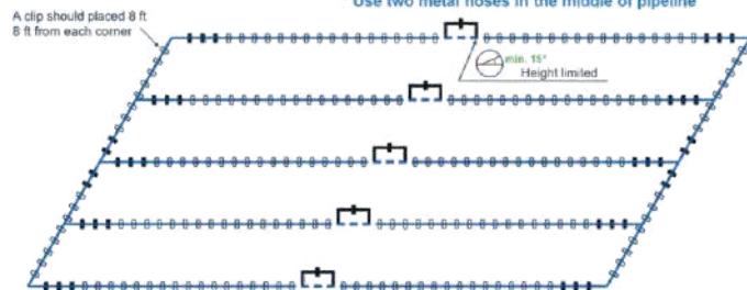
B2) Multiloop pipeline for DN150-DN200 * Use two metal hoses in the middle of pipeline
