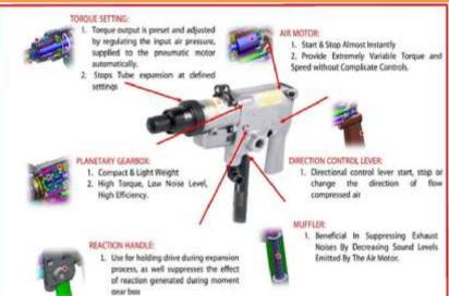
Areas where sparking tools are not allowed, Pneumatic Rolling Drives are the best choice for tube expansion. Its precise tripping mechanism makes it a highly accurate tool for tube expansion.
