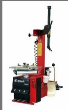
Semi Automatic S622 Tyre Changer Machine
