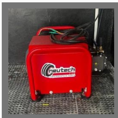
150 Bar Three Phase High Pressure Washer
