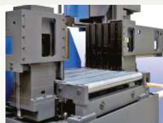
Hydraulic Auto indexing shuttle with much wider & heavy vices to pull heavy loads and synchronized with auto cycle
