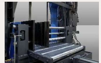
Heavy duty Auto Indexing Shuttle with much wider & Vices for Rigid Clamping of the Heavy Jobs for smooth indexing without Slippage.
