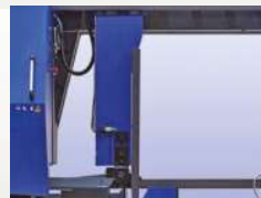
Automatically Adjustable, Dove-tail Type Heavy Duty Movable Blade Guide with hydraulic locking facility.
