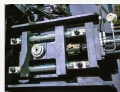
State of the art Four Point Pillar Type Hydraulic Blade Tensioning
