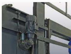
High efficiency power transmission to Saw through PLANETARY GEAR BOX
