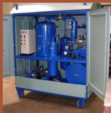
Transformer Oil Filtration
