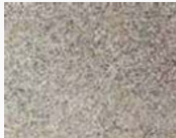
SSPC-SP-6 SA 2 NACE 3 3rd Quality Steel Structures Painting Council (USA) Swedish Standards Organization National Organization of Corrosion Engineers (USA) United Kingdom Standards (BS 4232)
