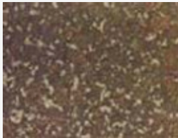
SSPC-SP-7 SA 1 NACE 4 Steel Structures Painting Council (USA) Swedish Standards Organization National Organization of Corrosion Engineers (USA)
