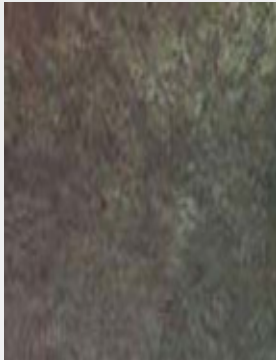
Steel surface largely covered with adhering mill scale but little, if any, rust.
