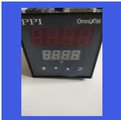
PPI Omnix ( Single Set Point Temperature Controller with Programmable Input/Output )
