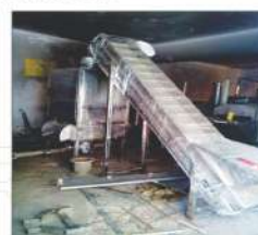
ONLINE HYDRO WITH CONVEYOR
