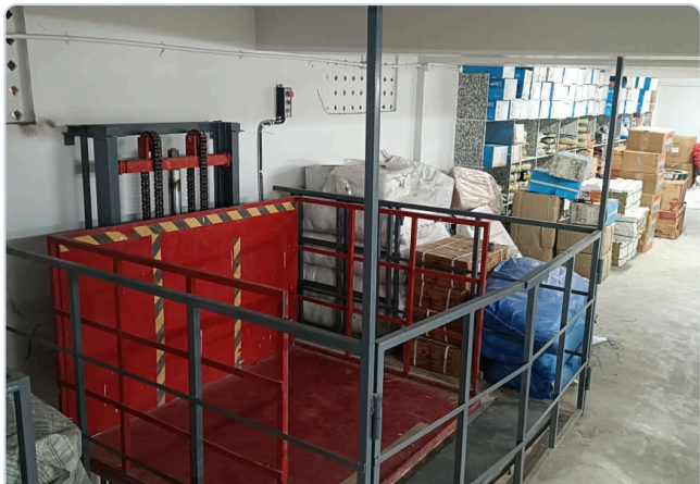
Fig 1.2: Caged Cargo Platform with Safety Railings
