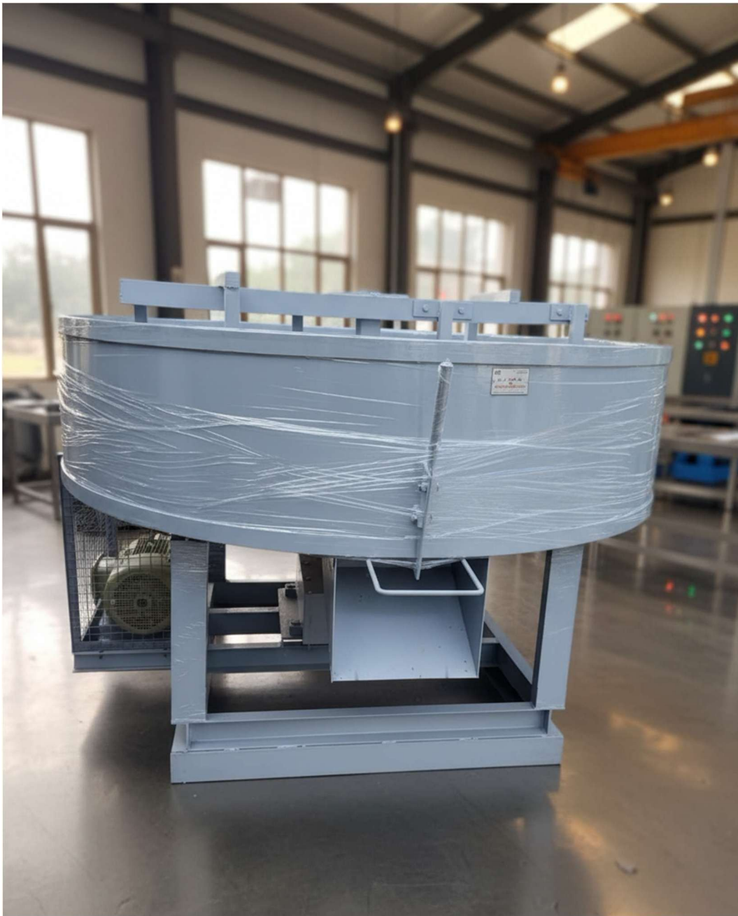
Mixer Machine (1200mm × 20 inch, 5 HP)
