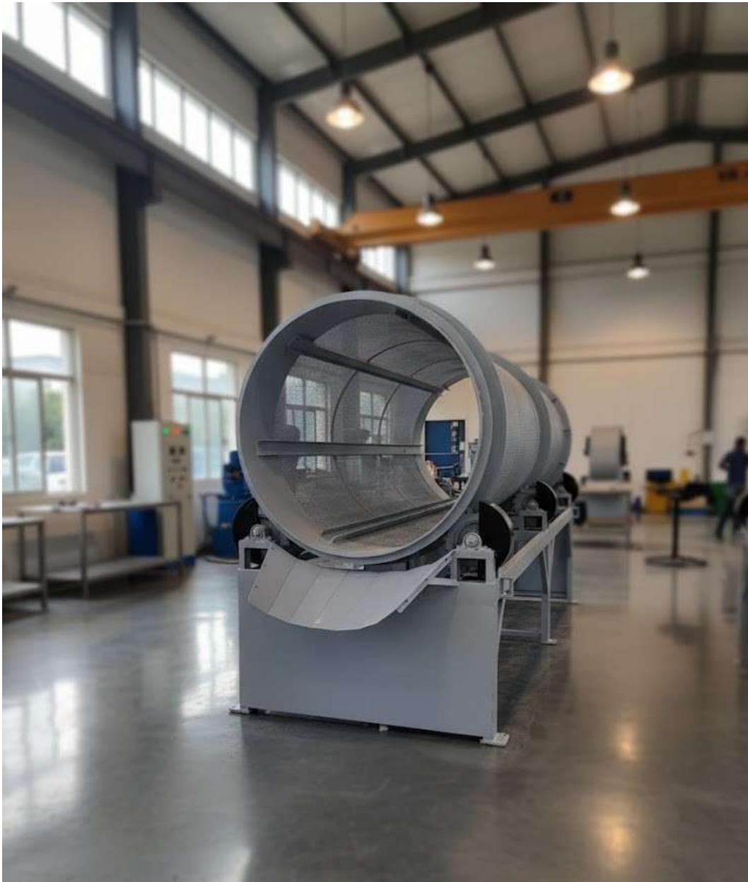
Trommel Screening Unit (2 ft × 8.5 ft, 2 HP Geared)
