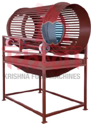
MODEL : GRADER CAP : 4000 KG P/H ELE : 1.5 HP
