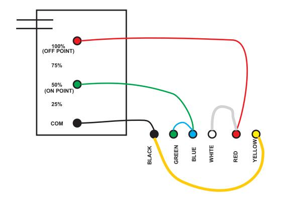
If Sensors are Not installed in sump Just inter connect all the wires as shown
