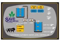
For Both Sump & Bore **Protections: Low & High Voltage** Dry Run, Sump Low, Delay ON
