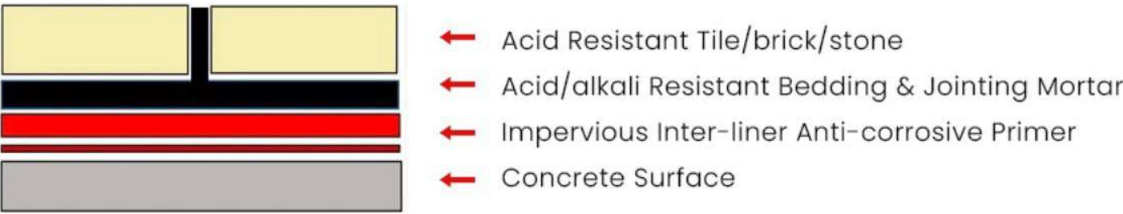
DESIGN VIEW FOR ACID RESISTANT BRICK/TILE LINING THE MEMBRANE BRICK/TILE/STONE LINING
