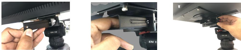
Pick up the Clip , and insert in the Base ( from where it was taken out ) , insert the Wing screw from the Monitor Mounting Clip to the the clip inserted first and tighten screw as per the monitor position needed .
