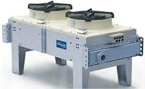
The transformer oil cooler is used to cool power transformers by means of forced air and oil flow. The oil in the cooler is circulated using a pump.
