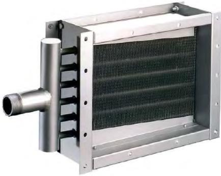
**Steam coils** are manufactured from thick walled copper tubes and heavy gauge copper headers with flow drilled holes for a strengthened joint.
