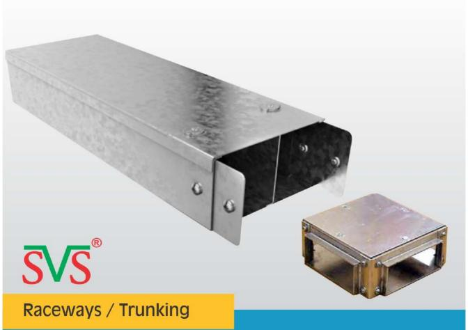
Cable Trunking is used primarily for light duty applications like data cables, telecommunications, control cables. These are Solid Bottom Trays provided with Cover & either are compartmentalised or not depending on site conditions. Raceways are enclosed from all sides to protect cables from sunlight, falling objects, dust and water or other liquid.
