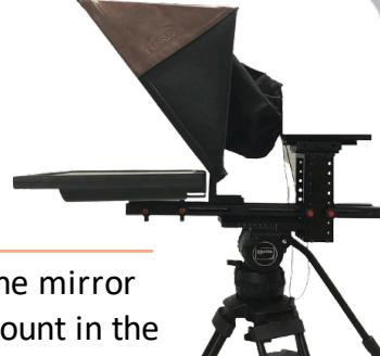
Take the Hood and put it on the mirror frame + Insert the Camera Mount in the Base and adjust with screws
