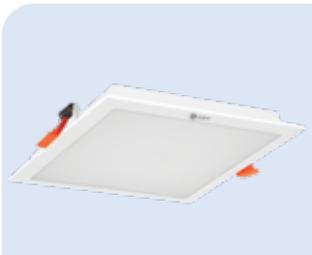
Recess-mounting low-height square LED downlighter designed with excellent thermally managed aluminium pressure die-cast housing with heat-dissipating fins for larger surface area, finished in epoxy powder-coated white.
