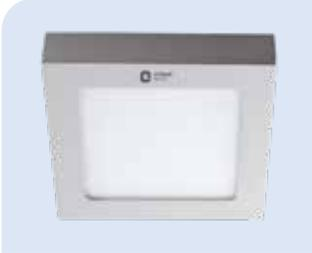
Ultra slim surface-mounting square LED downlighter designed with excellent thermally managed aluminium pressure die-cast housing with heat-dissipating fins for larger surface area finished in epoxy powder-coated white to deliver high efficacy light output and uniformity, utilising edge-lit technology.
