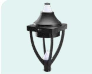
LED Post-top IP65 elegantly designed die-cast aluminium housing and high grade aluminum heat sink for efficient thermal management, sturdiness and excellent corrosion resistance. 4 nos. die-cast aluminium arms are provided to support the housing. Powder coated black after phosphochromate treatment.
