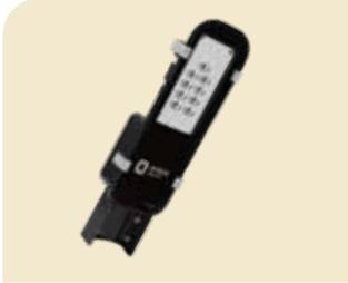
Highly efficient IP66 LED street-light with aluminium pressure die-cast housing, toughened glass in the front and peanut lens for batwing light distribution, higher spacing between poles and maintenance-free system.
