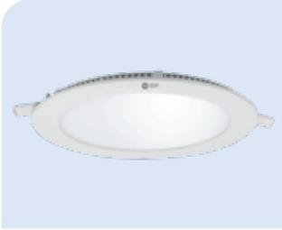
Ultra slim recess-mounting round LED downlighter designed with excellent thermally managed aluminium pressure die-cast housing with heat-dissipating fins for larger surface area finished in epoxy powder-coated white to deliver high-efficacy light output and uniformity, utilising edge-lit technology.
