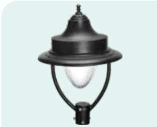
LED Post-top IP65 designed in spun aluminium housing and excellent corrosion resistance. 2 nos. aluminium arms are provided to support the housing. Powder coated black after phosphochromate treatment.
