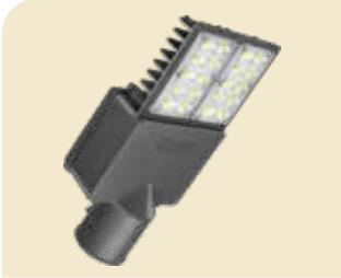
Highly efficient IP66 LED streetlight with high-power LEDs; having aluminium pressure die-cast housing and PC cover in the front and lens for batwing light distribution.
