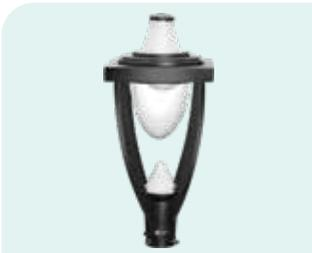
LED Post-top IP65 elegantly designed die-cast aluminium housing and high grade aluminium heat sink for efficient thermal management, sturdiness and excellent corrosion resistance. 4 nos. die-cast aluminium arms are provided to support the housing. Powder coated black after phosphochromate treatment.
