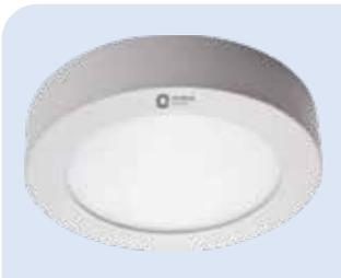
Ultra slim surface-mounting round LED downlighter designed with excellent thermally managed aluminium pressure die-cast housing with heat-dissipating fins for larger surface area finished in epoxy powder-coated white to deliver high-efficacy light output and uniformity, utilising edge-lit technology.
