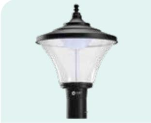
LED Post-top IP65 elegantly designed spun aluminium and high grade aluminium heat sink for efficient thermal management, sturdiness and excellent corrosion resistance. MS base provided to support the housing. Powder coated black after phosphochromate treatment.
