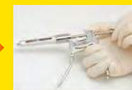
When releasing it after use, push Release and pull Rod lever to remove the ampoule.
