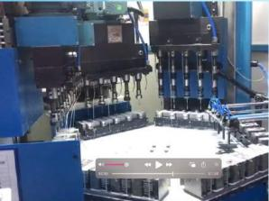
Multi Spindle Drilling And Tapping Machine with Rotary Table
