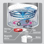
Pigments which are going to settle at the bottom of ink reservoir will be stirred from top to bottom by the stirrer.
