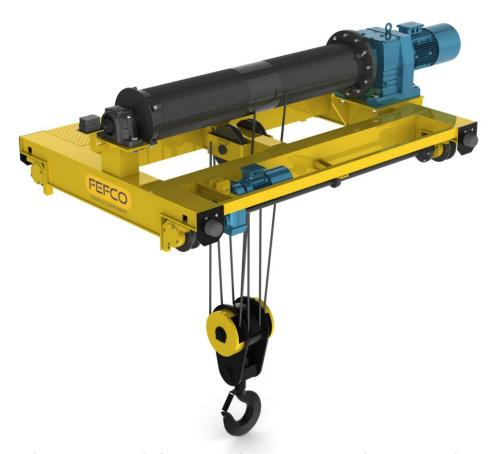
A compact designed crab unit for the various load capacity range, with articulated end carriage joints ensuring positive contact of all four wheels with the track, with two direct drive cross travel motors. Load capacity range: It to 50t
