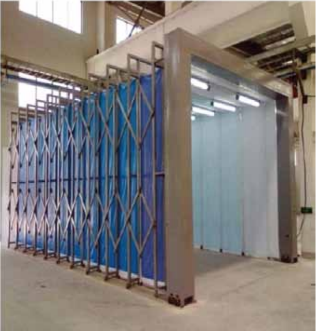
Movable Paint Booth
