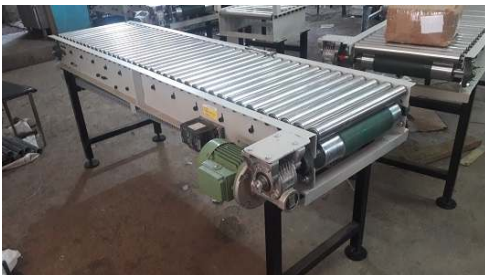
Rollers driven by PVC belt
