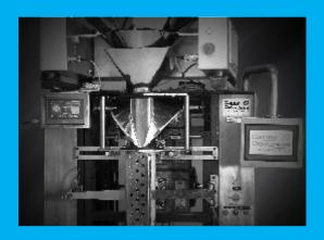
Un common shaped forming caller increases the paper stability & allows paper to shape itself improving the sealing finishing & strength.
