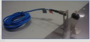
the vent opens, the magnet element will move away from the reed switch and an alarm signal is initiated to shutdown the process or to generate a trouble condition.
