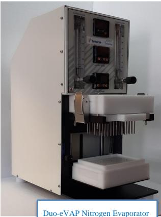
Evaporates Single 96 Well Plate -For aqueous or organic solvents (not dry or concentrated acid solutions)
