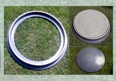
GRP manhole covers which are made from composite material such as glass fiber, resin, and quartz so on. GRP Manhole cover is lightweight and excellent protection against corrosion and the effects of chemicals because it is made from FRP (fiber reinforced plastic). It weighs only one seventh of the weight of an average cast iron cover. Because this cover is lightweight, it is easy to remove it during maintenance.
