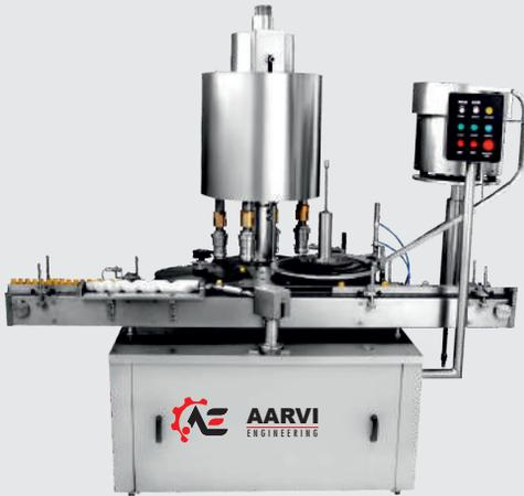
**Automatic Screw Capping Machine** is versatile, high efficient & compact model. The **AESC 60/100/150/200** model is suitable for capping of pre-threaded cap on various sizes of bottle.
